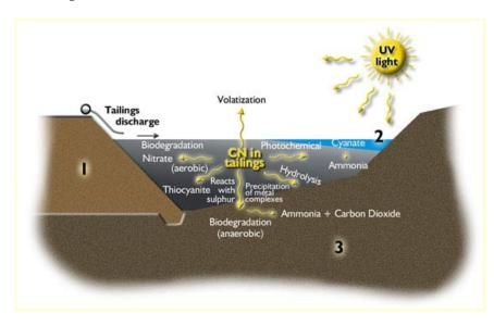
After discharge, the water is circulated back into the process; the decant water in the TMF during the entire period of storage, is subject to passive treatment processes, including natural degradation of the cyanide, hydrolyses, volatilization, photo-oxidation, bio-oxidation, mixing / separation, adsorption, dilution due to rainfalls etc.
