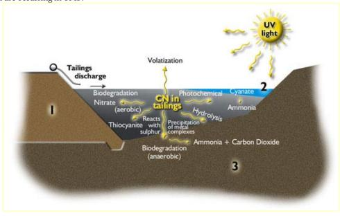
After discharge, the water is circulated back into the process; the decant water in the TMF during the entire period of storage, is subject to passive treatment processes, including natural degradation of the cyanide, hydrolyses, volatilization, photo-oxidation, bio-oxidation, mixing / separation, adsorption, dilution due to rainfalls etc.
