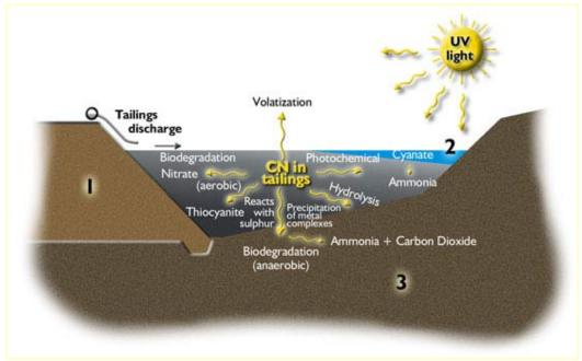
degradation/decomposing processes which the CN goes through, once discharged into the TMF.
