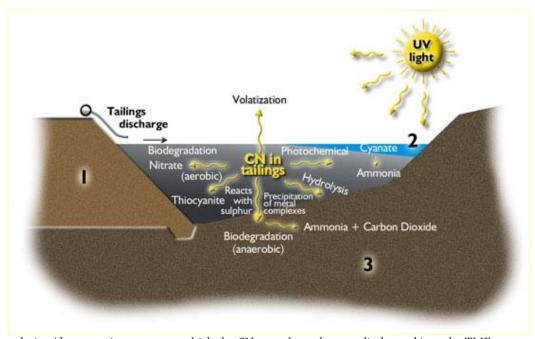
degradation/decomposing processes which the CN goes through, once discharged into the TMF.
