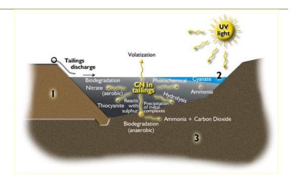
After discharge, the water is circulated back into the process; the decant water in the TMF during the entire period of storage, is subject to passive treatment processes, including natural degradation of the cyanide, hydrolyses, volatilization, photo-oxidation, bio-oxidation, mixing / separation, adsorption, dilution due to rainfalls etc.
