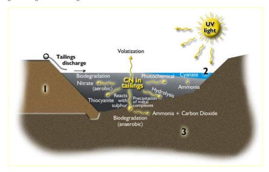
After discharge, the water is circulated back into the process; the decant water in the TMF during the entire period of storage is subject to passive treatment processes, including natural degradation of the cyanide, hydrolyses, volatilization, photo-oxidation, bio-oxidation, mixing / separation, adsorption,
