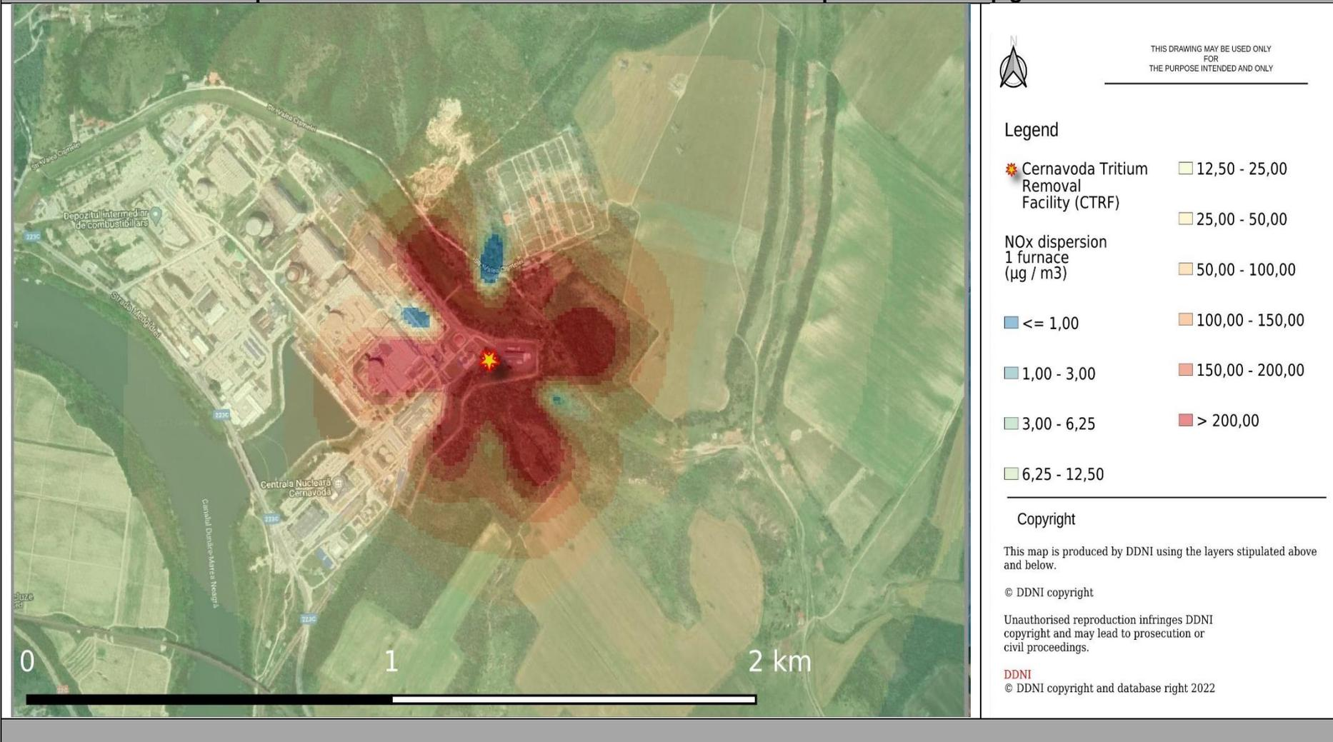
Spatial distribution of NOx concentrations under simultaneous operation of the 2 diesel units - back-up generator
