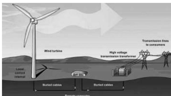
**Figure 14.** *The principle of complex and functioning of the wind farm*
