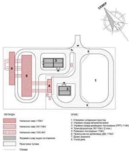
**Figure 18.** Complex and organization of the 110/35 kV substation and the administrative building of the wind farm Kostolac
