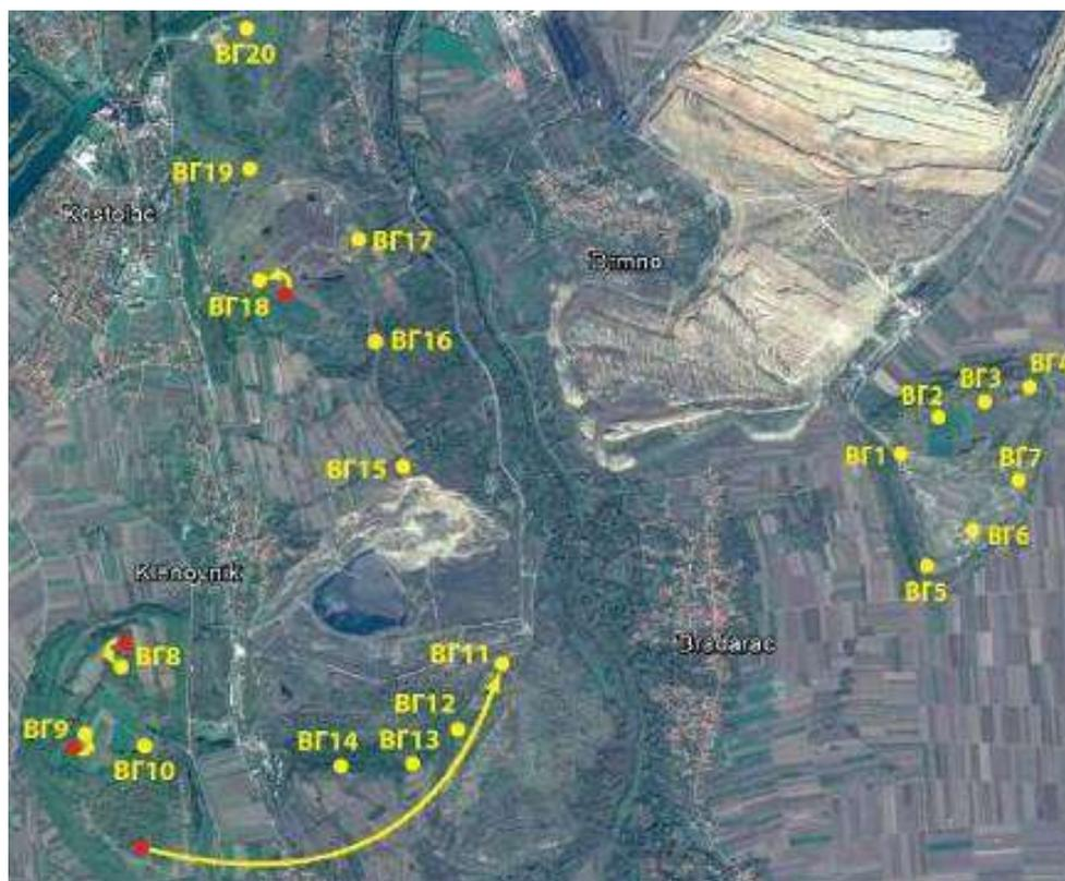
**Figure 20.** Changes in the spatial disposition of the wind turbines as a result of the analysis of potential conflicts with the flying fauna (red - the position of the wind generators according to GD, yellow - the position of the wind turbines after the conducted monitoring of the flying fauna)
