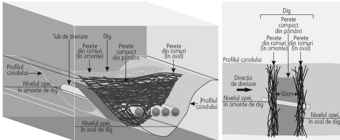
**Figure 2.** Diagram of a mixed dam constructed from natural and artificial materials (original)
