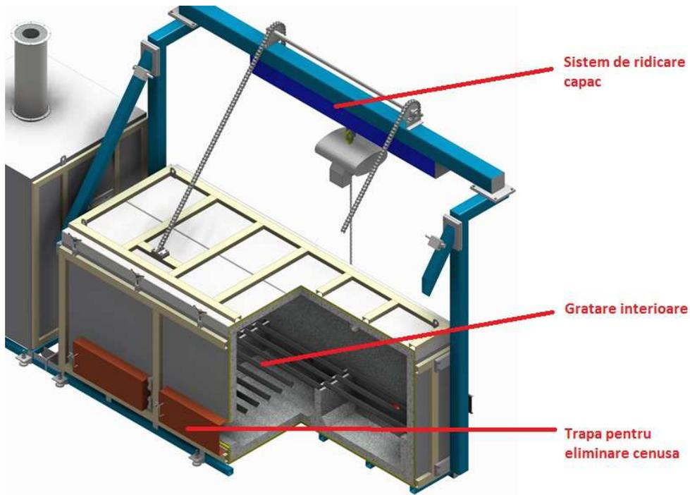
2. After burner chamber-it consists of a steel casing of the resistance anodized 5mm high temperatures padded, inside with refractory cement 8-10 cm. This room is equipped with:
