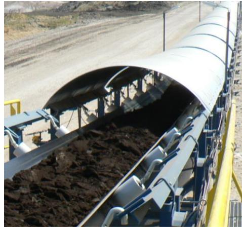
**Figure 3.3.4-7: An example of the system developed for covering the conveyor (conveyor for crushed coal in TPP Stanari)**
