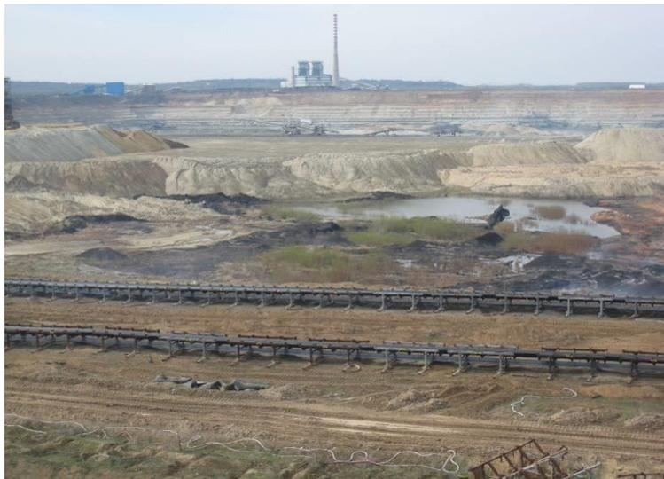
**Figure 2.8-3: Open cut mine Drmno - level of groundwater found at the bottom of the mine**
