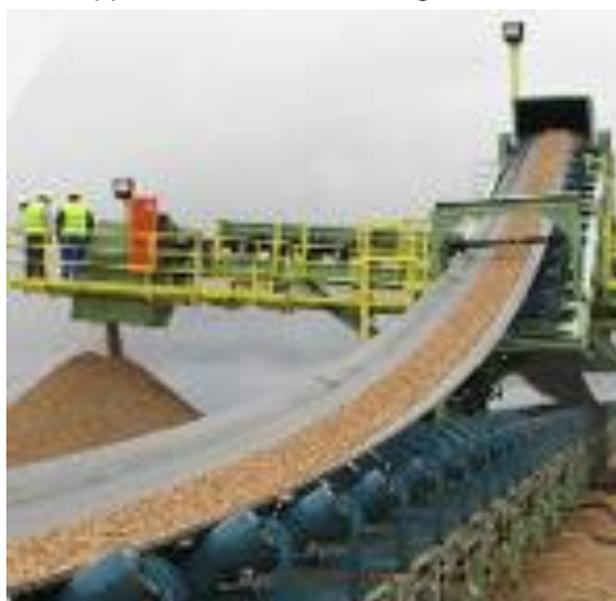
**Figure 3.3.4-11: Tripper car with discharge belt**
