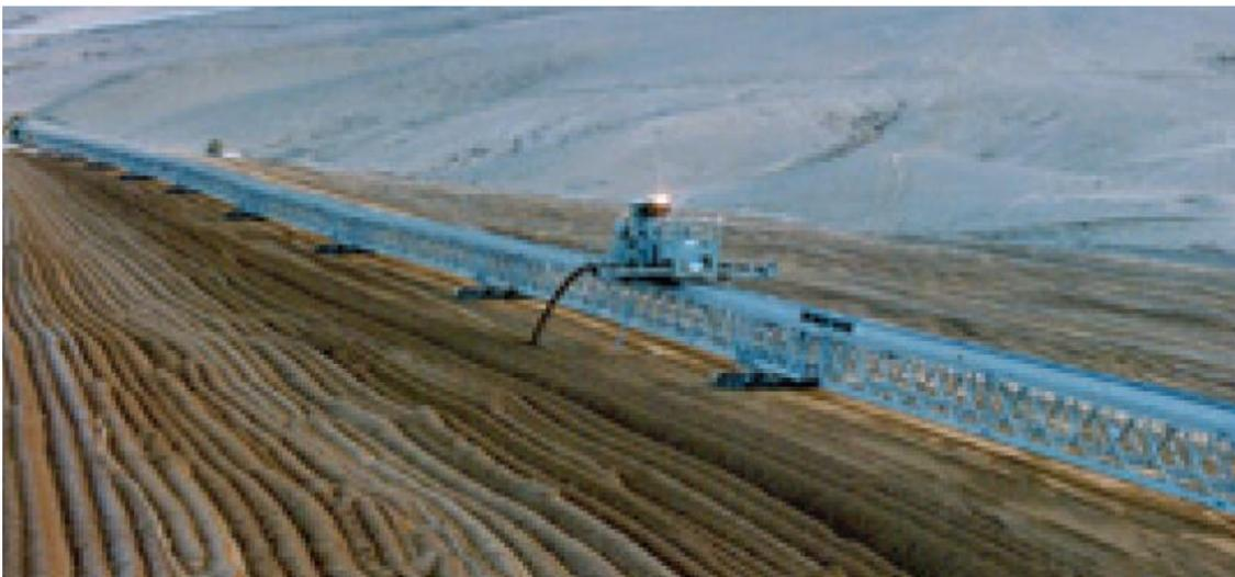
**Figure 3.3.4-10: Spreading conveyor belt with tripper car**
