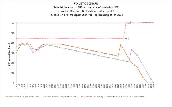
Figure 1b. Material balance of SNF stored in SFP-5 and SFP-6 in the Realistic scenario.
