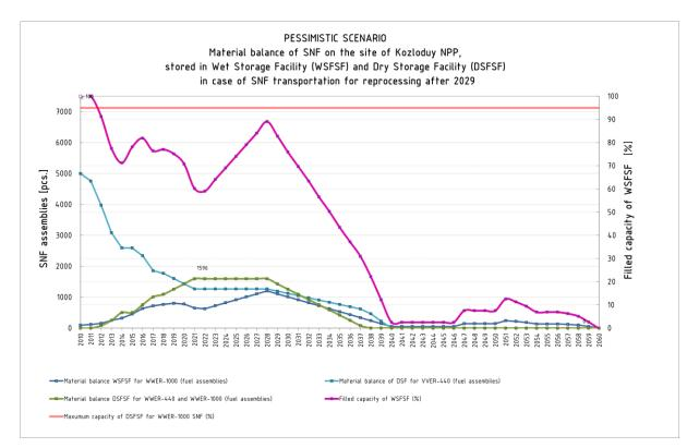
Figure 2a. Material balance of SNF stored in SFSF and DSFSF in the Pessimistic scenario.
