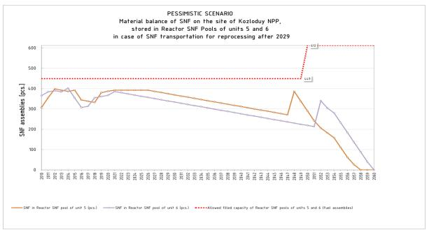
Figure 2b. Material balance of SNF stored in SFP-5 and SFP-6 in the Pessimistic scenario.
